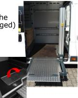
The lift is now ready to use. You can move the lift up and down with the button or with a remote controller.
